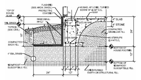
Figure 1: Initial foundation design at Ft. Drum (waiting for updated detail from Actus.)
